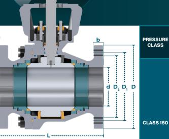
ASME B16.10 Face to Face | API 16.5 Flange API 607 | API 608 | NACE Cryogenic Options Available
