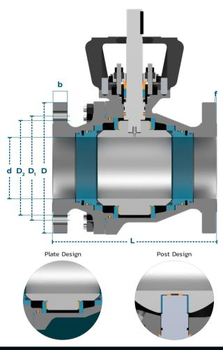
All designs, materials and specifications are subject to change without notice. Dimensions shown are full port "long pattern" design. Internal Trunnion plate Design for size 4" and above.
